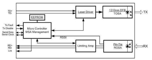
The module operates by a single +3.3V power supply. LVCMOS/LVTTL global control signals, such as Tx\_Fault,Tx\_Disable, are available with the modules. The SFP28 ER IT module electrical interface is compliant to 25GAUI and CEI-VSR-28G-VSR. It has been designed to meet the harshest external operating conditions including temperature, humidity and EMI interference. The module
