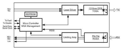
This 25Gb/s SFP28 LR BiDi transceiver is designed to transmit and receive optical data over 10km single modeoptical fiber.
