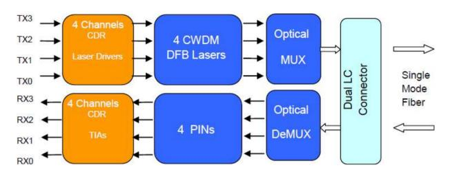
This product is a transceiver module designed for 2km optical communication applications. The design is compliant to 1000GBASE CWDM4 MSA standard. The module converts 4 inputs channels (ch) of 25Gb/selectrical data to 4 CWDM optical signals, and multiplexes them into a single channel for 100Gb/s optical transmission. Reversely, on the receiver side, the module optically demultiplexes a 100Gb/s input into 4 CWDM channels signals, and converts them to 4 channel output electrical data.
