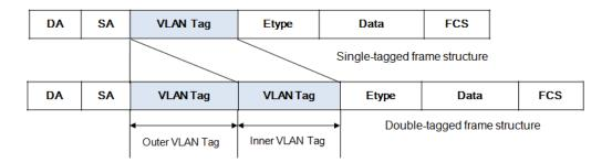
The port QinQ feature is a flexible, easy-to-implement Layer 2 VPN technique, which enables the access point to encapsulate an outer VLAN tag in Ethernet frames from customer networks(private networks), so that the Ethernet frames will travel across the service provider's backbone network (public network) with double VLAN tags. The inner VLAN tag is thecustomer network VLAN tag while the outer one is the VLAN tag assigned by the service
