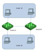
A VLAN can span across multiple GPONes, or even routers. This enables hosts in a VLAN to be dispersed in a looser way. That is, hosts in a VLAN can belong to different physical networksegment. Compared with the traditional Ethernet, VLAN enjoys the following advantages.
