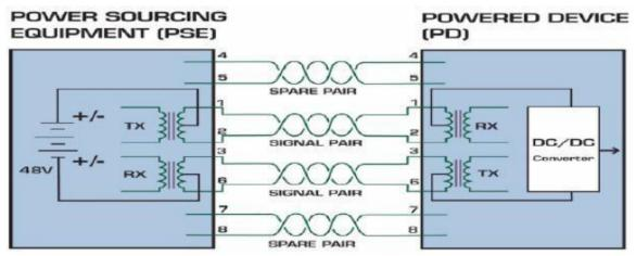
Generally speaking, standard PD has to support two power reception modes, while PSE only needs to support one of the two modes. All products, as the PSE switches, only support the signal line power supply—alternative A.
