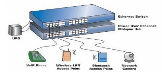
Meanwhile, 802.3af Standard also defines the PI (Power Interface: The interface between PSE/PD and network cable). At present, two power supply modes: Alternative A (Signal line No. 1, 2, 3, 6) and Alternative B (Free line 4, 5, 7, 8), have been defined, which are described as follows: 1) Supply the power through the idle pairs — Mode B (Alternative B)
