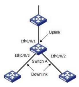
As shown in the figure, ports GigabitEthernet 0/0/1, GigabitEthernet 0/0/2, and GigabitEthernet0/0/3 of GPON A form a monitor link group.
