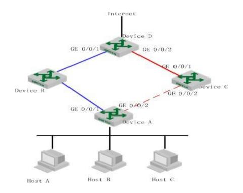
To avoid traffic interruption due to the failure of the link on which GigabitEthernet 0/0/1 of GPON B resides, configure a monitor link group on GPON B, and specify GigabitEthernet 0/0/1 as the uplink port, and GigabitEthernet 0/0/2 as the downlink port.
