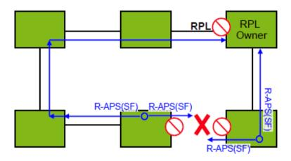
when the link of the faulty device recovers, it sends RAPS (NR) packets to other devices in the ring to inform them that there is no local request. When the RPL owner receives the packet, it will block the port and send the R-APS (NR, RB) message again after some time. After receiving the packet, the other nodes will refresh the FDB entry. Later, the port of the faulty node will be restored to the forwarding state, and the ring will revert to the IDLE state.
