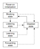
When you power up the Switch, spanning tree is enabled by default, and every interface in the Switch, VLAN, or network goes through the blocking state and the transitory states of listening and learning. Spanning tree stabilizes each interface at the forwarding or blocking state.
