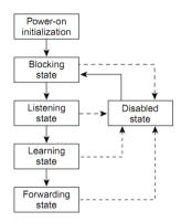
When you power up the GPON, spanning tree is enabled by default, and every interface in the GPON, VLAN, or network goes through the blocking state and the transitory states of listening and learning. Spanning tree stabilizes each interface at the forwarding or blocking state.
